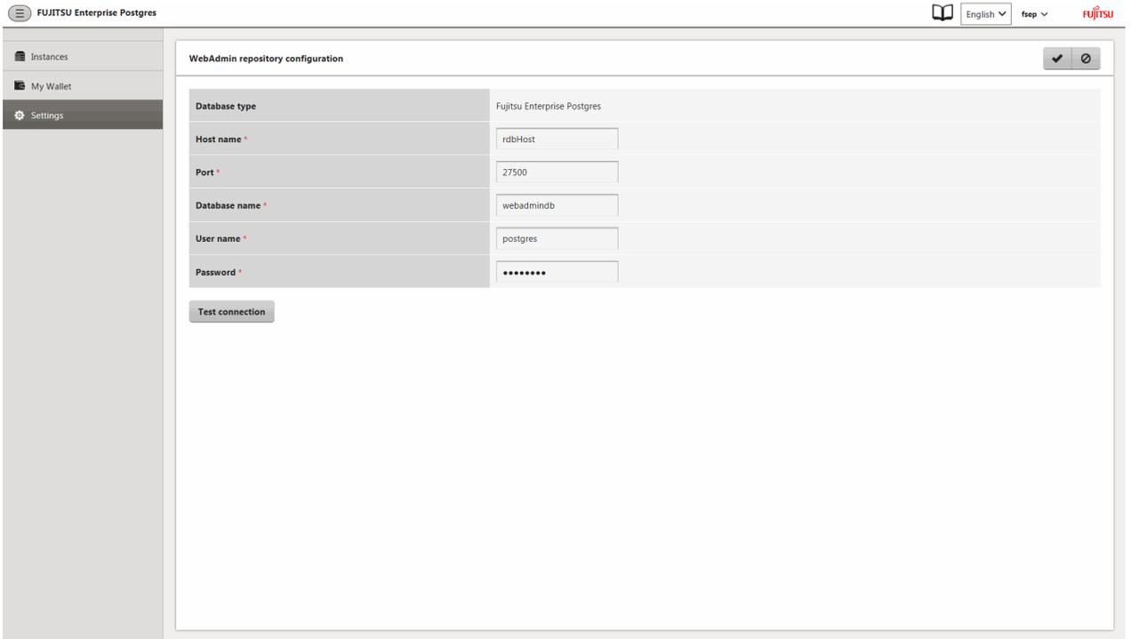
The screenshot shows the 'WebAdmin repository configuration' page in the Fujitsu Enterprise Postgres interface. The page has a sidebar on the left with 'Settings' selected. The main content area contains a configuration form with the following fields:
