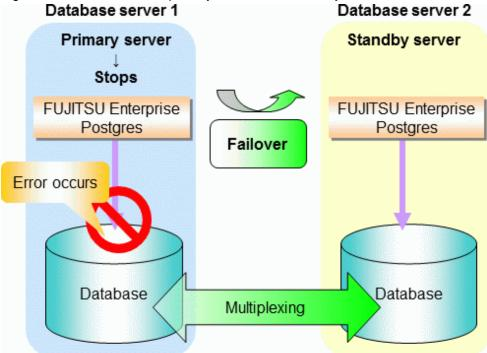
Figure 2.2 Standby server disconnection
