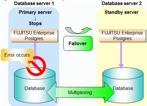
Figure 2.2 Standby server disconnection
