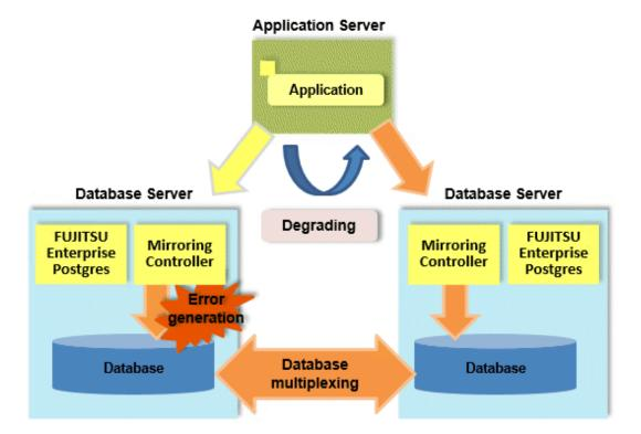
FUJITSU Enterprise Postgres not only mirrors a database using the PostgreSQL streaming replication feature, but also provides simplified switchover and standby disconnection features as well as a feature to detect faults in elements that are essential for the continuity of database process, disk, network, and other database operations.
