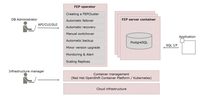
This operator will deploy a standalone as well as highly available FUJITSU Enterprise Postgres cluster with pre-defined configuration to get started with small workload. User can adjust the configuration parameters at the time of deployment and after to make the instance suitable for the workload.
