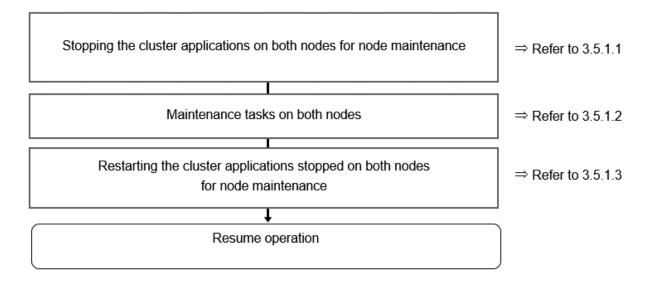
Figure 3.2 Workflow for mutual switch maintenance
