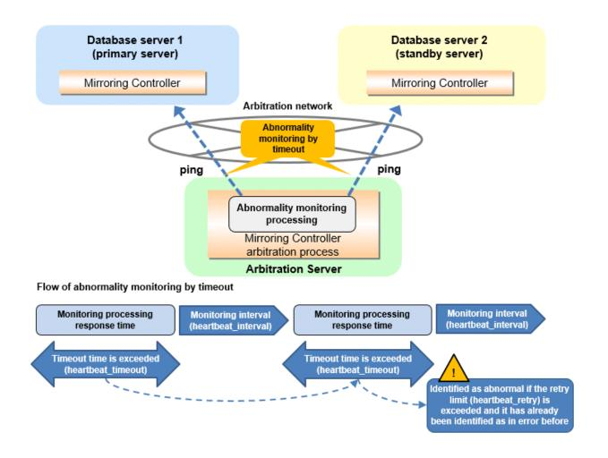
The expression for calculating the time required to detect an abnormality by Mirroring Controller arbitration process is shown below.
