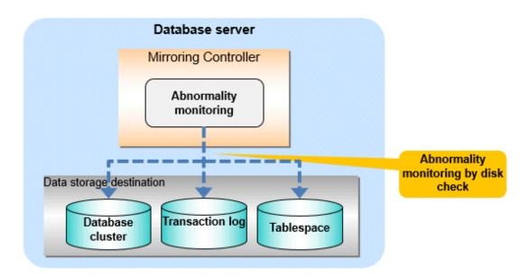
In disk error monitoring, a disk check is performed, and degradation is performed when an error is first detected within the error detection time or the time set in disk\_check\_timeout. However, in order to disconnect the standby server when disk\_check\_timeout detects an error on the standby server, shutdown\_detached\_synchronous\_standby must be set to on.
