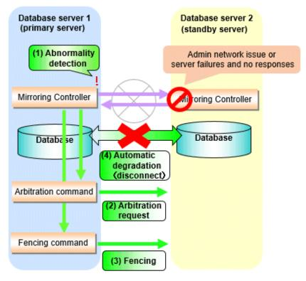
Database server 1 Database server 2 (standby server) (primary server) (1) Abnormality Admin network issue or detection server failures and no responses Mirroring Contro Mirroring Controller Database Da tabase (4) Automatic degradation (switch) Arbitration command (2) Arbitration request Fencing command (3) Fencing
