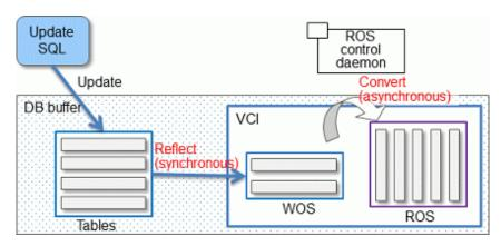
The same scan results can be obtained without a VCI by using WOS in conjunction with ROS. More specifically, WOS is converted to Local ROS in local memory for each aggregation process, and aggregated with ROS.
