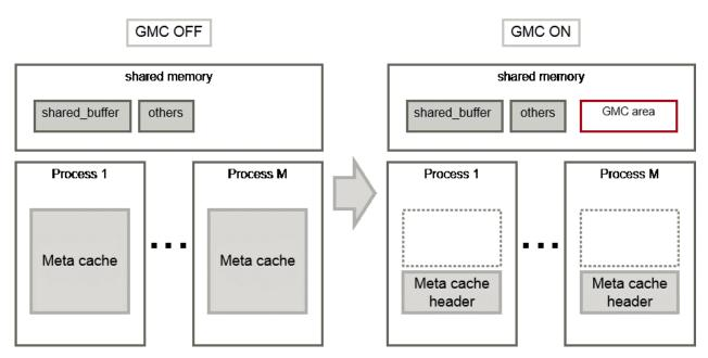
When the GMC feature is on, the per-process meta cache is cached in the GMC area on shared memory. Reference to the GMC area and process-specific work information is cached in the memory of each process. PostgreSQL process searches the meta cache for each process and accesses the GMC based on the reference information. If there is no reference information
