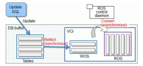
The same scan results can be obtained without a VCI by using WOS in conjunction with ROS. More specifically, WOS is converted to Local ROS in local memory for each aggregation process, and aggregated with ROS.
