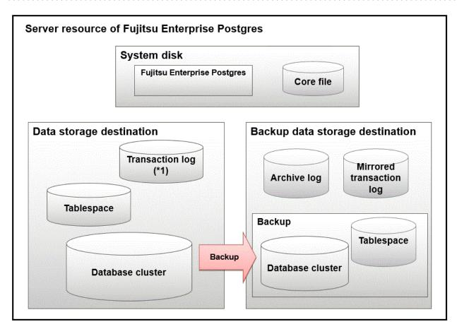
\*1: To distribute the I/O load, place the transaction log on a different disk from the data storage destination.
