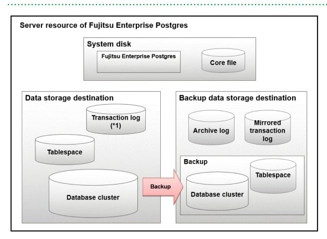
\*1: To distribute the I/O load, place the transaction log on a different disk from the data storage destination.
