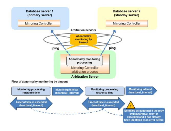
The expression for calculating the time required to detect an abnormality by Mirroring Controller arbitration process is shown below.
