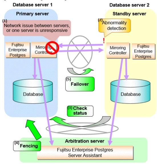
Figure 1.3 Database degradation using the arbitration server
