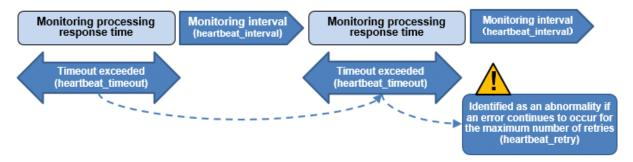
The expression for calculating the time required to detect an abnormality by Mirroring Controller is shown below.
