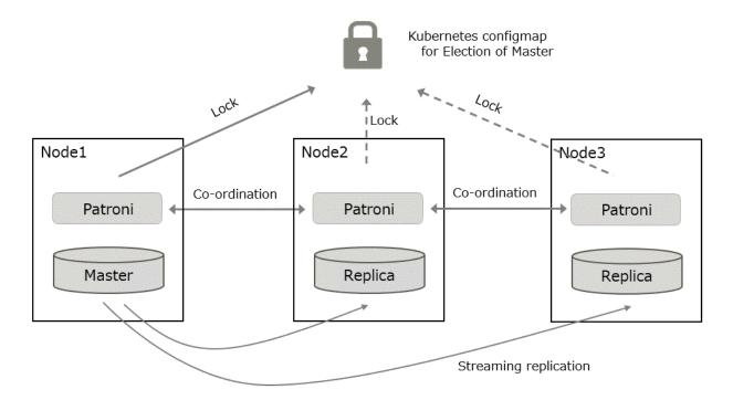
If Patroni detects a failure in the cluster, either because the Postgres process crashed or the container where Postgres is running dies, Patroni will initiate a failover automatically.
