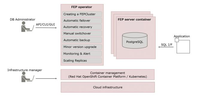
This operator will deploy a standalone as well as highly available Fujitsu Enterprise Postgres for Kubernetes provides automated operations for installing and managing your Fujitsu Enterprise Postgres 15 on OpenShift Container Platform or Kubernetes.
