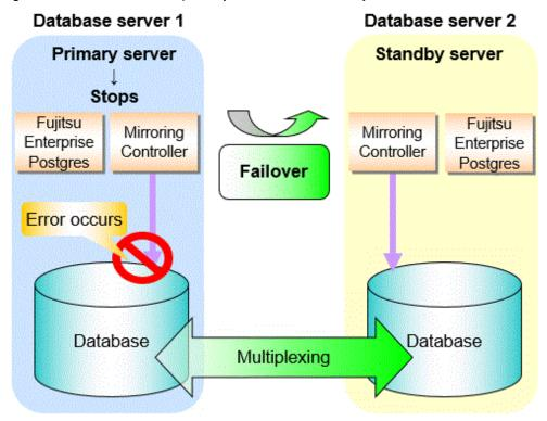
Figure 1.2 Standby server disconnection
