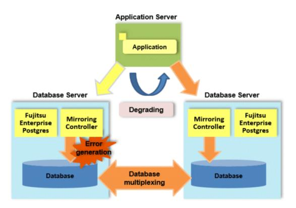
Fujitsu Enterprise Postgres not only mirrors a database using the PostgreSQL streaming replication feature, but also provides simplified switchover and standby disconnection features as well as a feature to detect faults in elements that are essential for the continuity of database process, disk, network, and other database operations.
