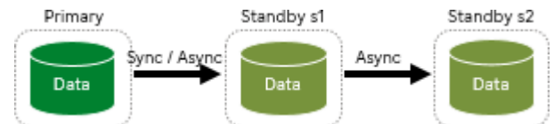
Active-passive database system (single master, single slave to cascaded slave(s))
