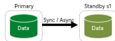
Active-passive database system (single master, single slave)
